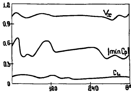
Fig. 17 Typical dependence of hydrodynamic characteristics of blade section at r = 0.7 on angle \theta
